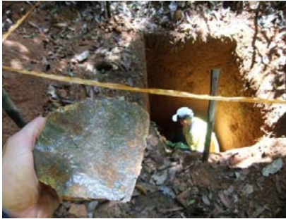
Trench sampling at Porto Grande uncovers widespread hematite and massive magnetite iron mineralisation.
